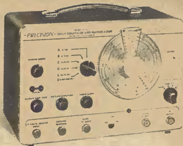
Model E-410C Sweep Generator/Marker Adder
